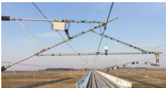
[Configuration of a dynamic state measurement system under high voltage and high current conditions]
