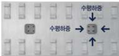
[Shear key horizontal support structure]
